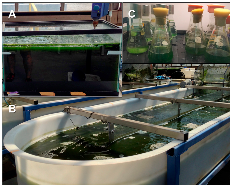
Figure 1. Large-, medium-, and small-scale vessels used in this study. This study used 100 L aquarium tanks as the medium-scale vessels (A), 1000 L raceway ponds as the large-scale vessels (B), and 0.25 L flasks as the small-scale vessels (C).
